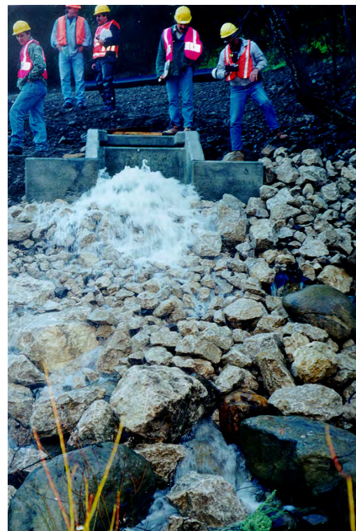
Testing of the upper Hilton Creek release point of the Supplemental Watering Facility.
